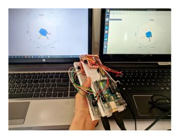
Figure 5: A prototype of the proposed solution. The orientations of the two devices are derived from the accelerometer and gyroscope data and are displayed in a simulated contactless payment.
